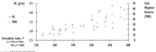
Figure G-34: Effect of Oxygen-Corrected Driveability Index on Driveability and Exhaust Emissions
