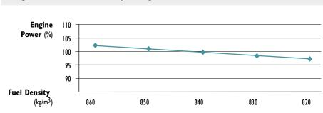
Figure DF-6: Effect of Density on Engine Power
