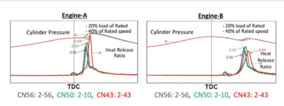
Figure DF-1: Cetane Number's Impact on Combustion in Two Engines
