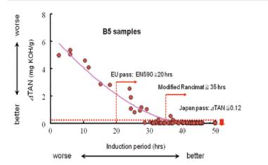
Figure DF-31: Correlation between Modified Rancimat Method and Delta TAN Method
