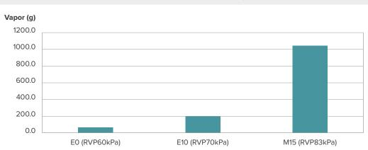
Figure G-26: Vapour Amounts from E0, E10 and M15 on CARB Running Loss Test (start fuel T = 35°C)
