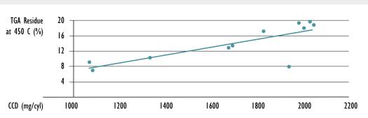
Figure G-52: Correlation of CCD and TGA Results of Commercial Fuels in Ford 2.3L IVD Test (ASTM D6201)
