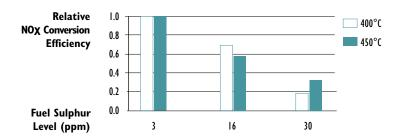
Figure DF-17: Effect of Fuel Sulphur Level on NOx Conversion Efficiency (150 Hours Aging)
