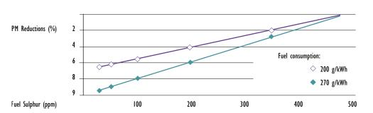
Figure DF - 11: Effect of Diesel Fuel Sulphur Level on PM Emissions Heavy-Duty Engines (PM = 0,10 g/kWh)
