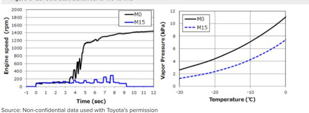
Figure G-25: Cold-Start Behaviour of M0 vs M15
