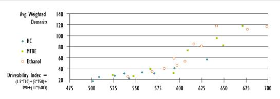
Figure G-33: Effect of Driveability Index (Oxygen Corrected) on Driveability
