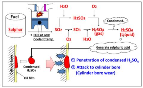
Figure DF-9: Mechanism of Sulphuric Acid Attack
