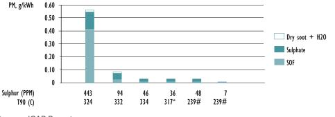
Figure DF-22: Fuel Effect on Diesel Particulate-CR (Continuous Regeneration) - DPF Japan Diesel 13 Mode
