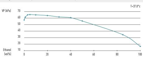
Figure G-36: Impact of Ethanol Level on Vapour Pressure at 37.8°C
